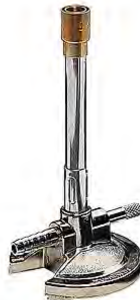
Figure 1. A “modern Bunsen burner, gas intake on the left, needle valve on the right, and air regulation around base. Public domain photo.
